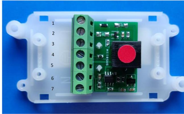
The Sensors, power and external alarm connect via a junction box which then connects via a single cable to the display unit.
